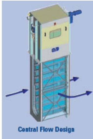
Figure 24 – Schematic of center fed band screen (Sketch courtesy of Bracket Green)
